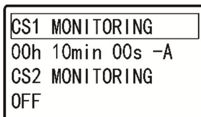
If monitoring function of one CS is shut down, the corresponding setting is OFF. If monitoring function of a CS is initiated, then the displayed setting is preset monitoring time value and monitoring level.
